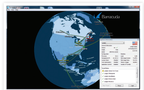
Barracuda Earth - the graphical real-time 3D network monitoring utility of the Barracuda Firewall Control Center, provides a status overview of all VPN site-to-site tunnels.
